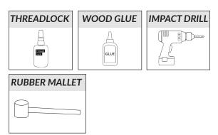
We strongly recommend applying thread lock to the full length of all screws, applying wood glue to the plugs and using an impact drill.
